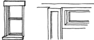
Window and parapet wall recesses and projections from wall surface to provide visual relief
