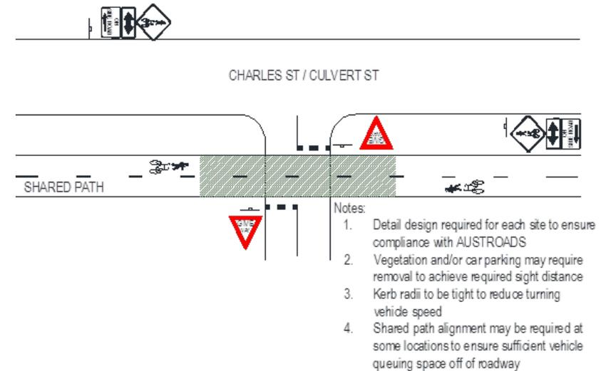
Figure 19: Changed priority - vehicles give way to shared path (typical example only).
