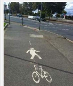
Photo 29: Section of footpath converted to shared path to access signalised crossing.
