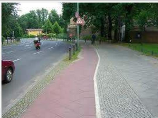
Photo 30: one-way separated path, Hamburg Germany (cycle path red paved / footpath (2-way) grey paved – separated by cobblestones).
