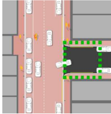
Temporary intersection closure
