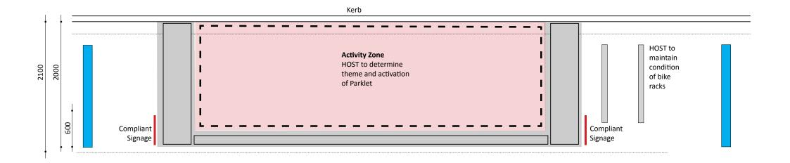
Buffer zone marked by ground mounted rubber wheel stop (By Council) Solid barrier end to enclose parklet resistant (By Council)
