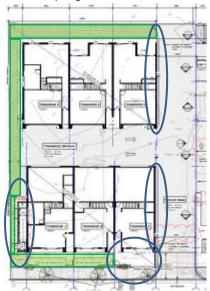
Opey Avenue ground level floor plan revision of layout and reduction of setback relief, including transformer room to street frontage.
