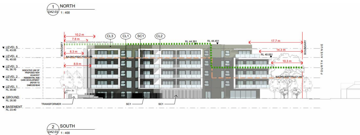
Figure 3-1 Building Envelope Diagram (TNVs orange line, Affordable Housing Incentive green line)
