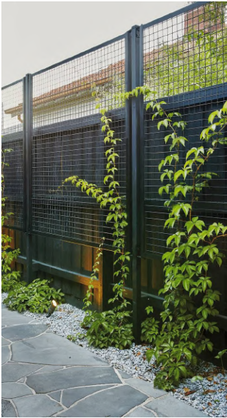
MS-POOL FREESTANDING METAL SCREEN. 3.2m HIGH 358 ANTICLIMB MESH. GALVANISED STEEL
