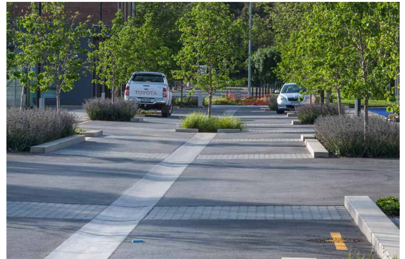
Bowden Urban Village, SA - Central planting, surface treatments and water sensitive urban design encourage quieter shared roadways.
