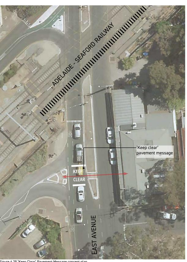
Figure 6.29 'Keep Clear' Pavement Message concept plan
