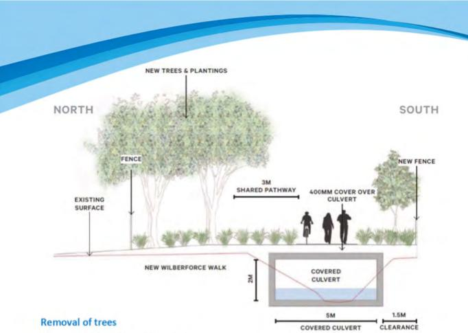
The early construction works require clearance of the creek channel including removal of the existing concrete channel and trees located within the corridor.
