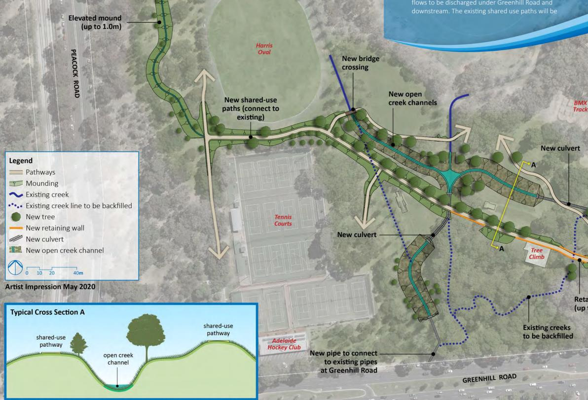
re-constructed to suit the new layout and the new drainage works will enable part of the existing creek alignment to be backfilled to support tree health. This section of the creek is in poor condition, and the red gums are vulnerable due to creek erosion.
